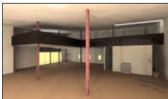
The RADIANCE daylight rendering program can show daylight penetration into a modeled room. This program can be used to predict the outcome of daylighting strategies when designing a building.
