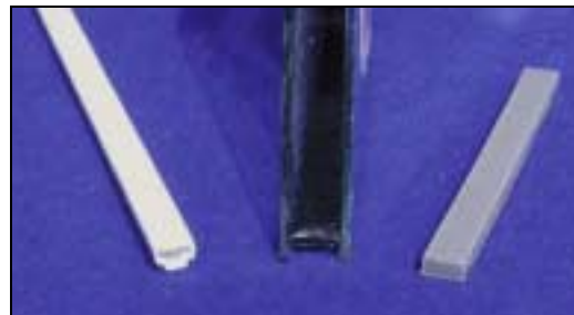
Left to right: Vinyl, Butyl-Rubber and Silicone-Foam Insulating Edge Spacers
