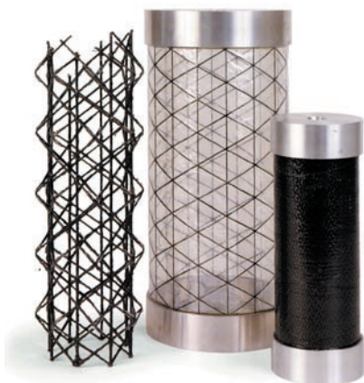
Lightweight collapsible carbon/ epoxy boom structures (McQuaid, 2005, 120)
