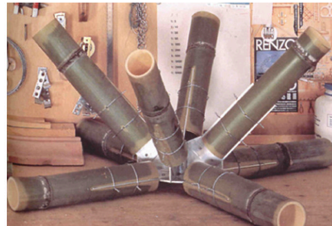
ILL.06 - Renzo Piano, bamboo steel connection
