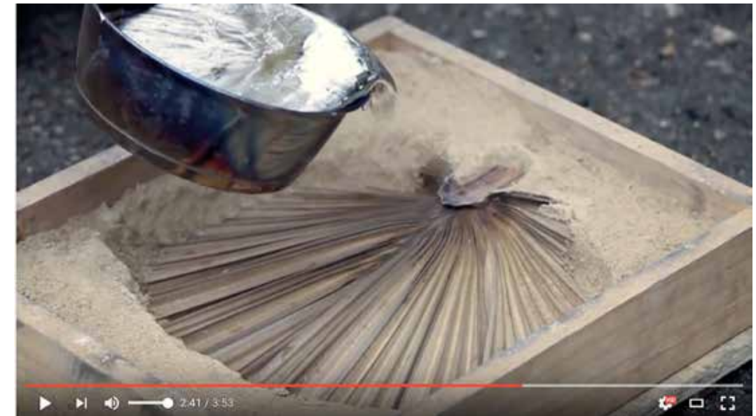
Fig. 89 - 2:41_Pouring in a first mould
