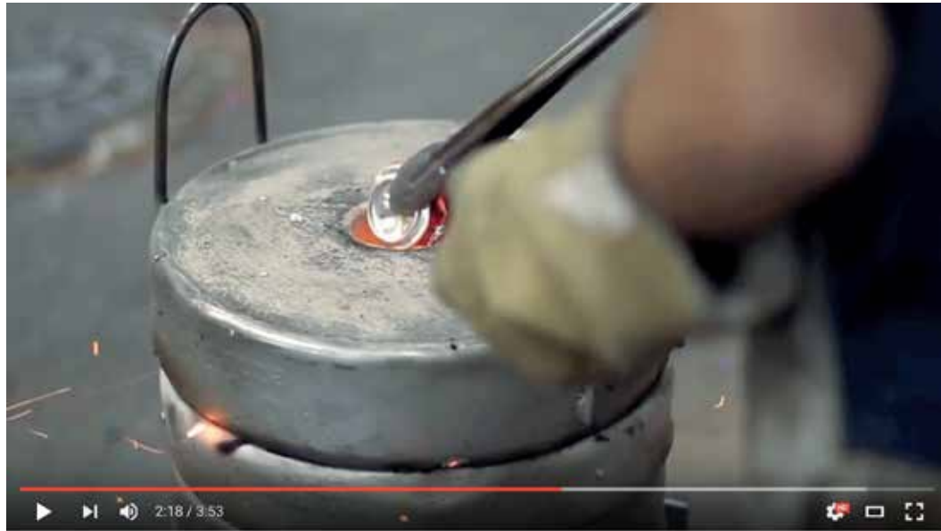
Fig. 83 - 2:18_Inserting the crushed cans in the furnace
