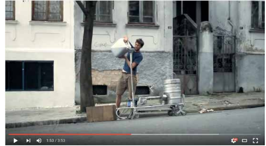
Fig. 78 - 1:53_Filling reservoir with collected used oil
