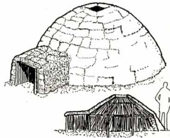
Figure 3.7: The summer house of the Nunamiut Eskimos follows the form of the igloo but is constructed using sticks covered with slabs of turf. (Redrawn from "Primitive architecture and climate," by Fitch and Branch. Copyright © 1960 by Scientific American, Inc. All rights reserved.)
