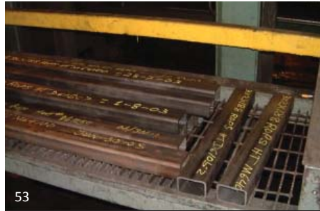
53 Fig. 2.2 One half standard fabrication tolerances are required for all elements to be incorporated into AESS 2 and higher.
