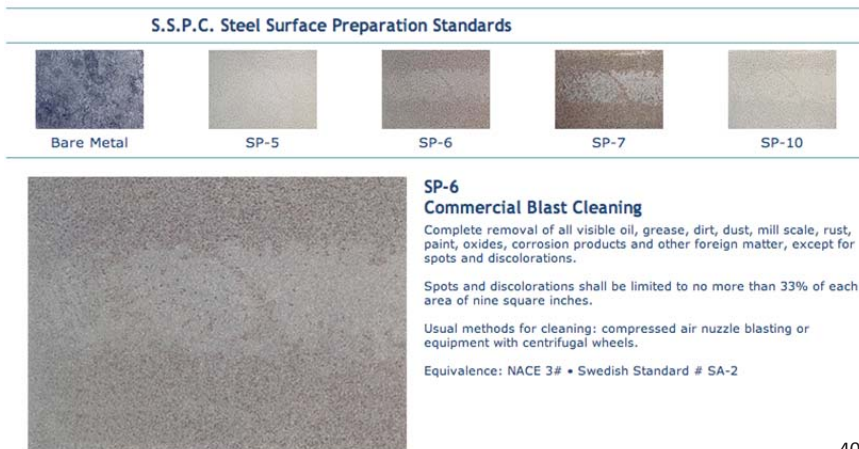
Fig. 1.1A Sample sheet showing the finish appearance for Steel Surface Preparation Standards. AESS starts assuming SP-6 finish. Image courtesy of Dry-Tec
