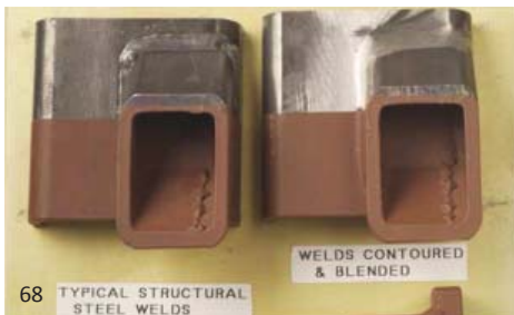
Fig. 4.2A Welds contoured and blended. The left hand sample shows typical structural welds. The right hand sample shows how they have been welded and contoured. Courtesy AISC
