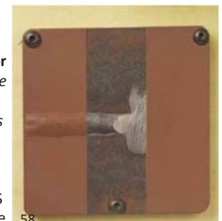
58 Fig. 3.2 Butt and plug welds ground smooth. Right side shows groove weld ground smooth. Courtesy of AISC
