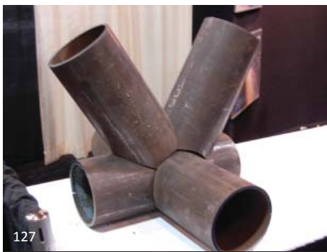
127 Modern equipment makes precision cutting of these intersecting round HSS members much simpler.
