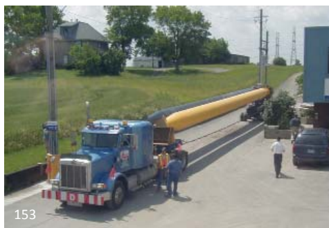
These pieces were so long that they could not fit on a normal trailer bed but were fitted with separate wheels on the back. This configuration also allowed for these extra long members to navigate around difficult corners.
