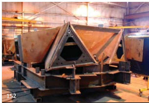
A temporary piece of steel joins the two points to stabilize the piece during shipping and erection.
