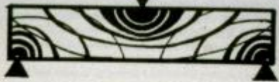
Light interference patterns showing stress in a plastic model beam under polarized light
