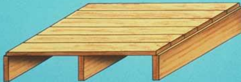
TWO SPAN CONTINUOUS PATTERN
